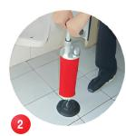
Push and press the handle up and down. Choose pressure by status of pipeline. 0~0.4~0.7Mpa
