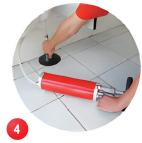
If there are some jam on top of the nozzle or the pipeline strait, join the air release extension pipe with the plug. Hole the plug by both hands and put out gas quickly.
